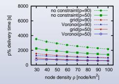
The speedup factor (i.e., the ratio of p%-delivery\_timewith and without mobility constraint) is approximately0.4 regardless of the node density and the value of pH. OhsakiCIF 201216/21
