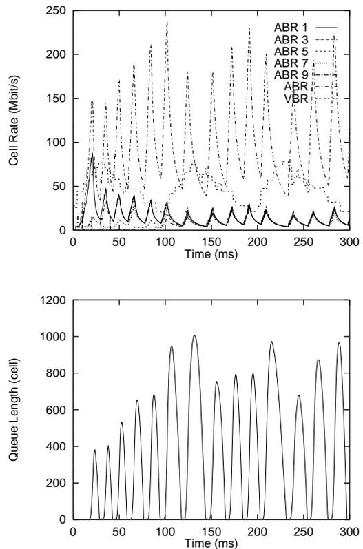
Fig. 6: Effect of VBR Traffic on EPRCA with an EFCI Switch ( $N_{VC} = 10, \tau = 1.00$ ).
