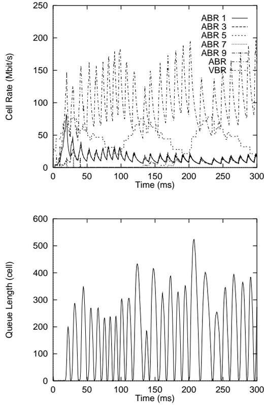
Fig. 7: Effect of VBR Traffic on EPRCA with a BES Switch ( $N_{VC} = 10, \tau = 1.00$ ).
