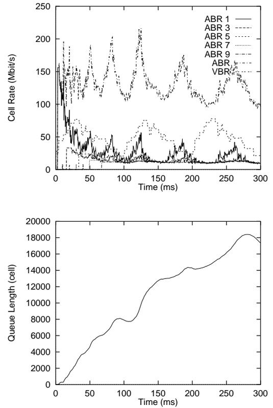
Fig. 9: Effect of VBR Traffic on EPRCA++ ( $N_{VC} = 10, \tau = 1.00$ , target utilization = 0.95).
