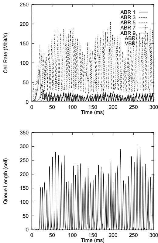
Fig. 8: Effect of VBR Traffic on EPRCA with an EDS Switch ( $N_{VC} = 10, \tau = 1.00$ ).
